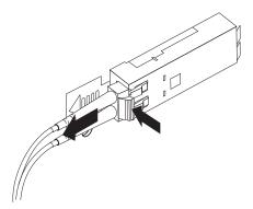
Figure 34. Removing the LC-LC Fibre Channel cable
